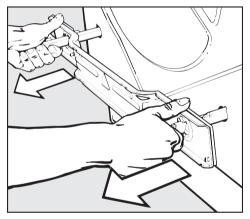
■ Withdraw the two struts together with the support plate.
